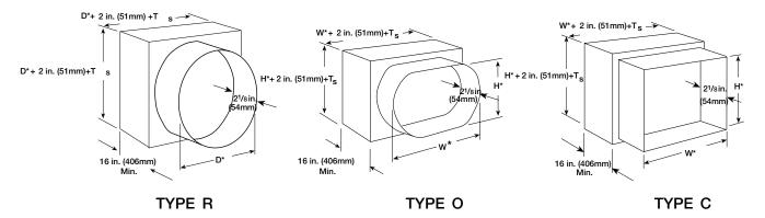
\* These dimensions are furnished approximately 1/4 in. (6mm) undersize, except round and oval dimensions which are approximately 1/8 in. (3mm) undersize. T<sub>S</sub> = (2)(Sleeve Thickness)
